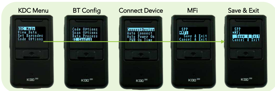
Figure 5 - Selecting a Bluetooth device type from the KDC menu
