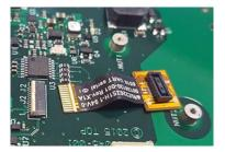
5. Replace the RS232 flex to ZIF cable with the USB flex to ZIF cable provided in the box and close the ZIF connector.
