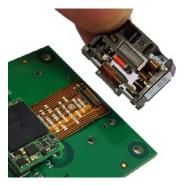
Note: Be sure the scan engine is right side up, the mounting holes should be facing the development board.
