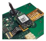
3. Disconnect the Mini DB from the flex to ZIF cable.
